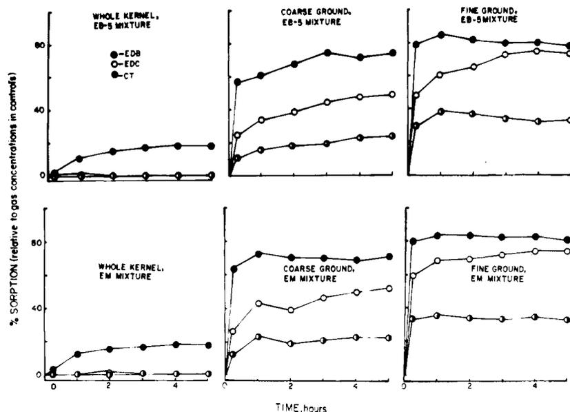
Figure 4. Sorption of ethylene dibromide, ethylene dichloride, and carbon tetrachloride in vapor phase at 27° C. by Selkirk wheat of 18.5% moisture content of three particle sizes and after two treatments
