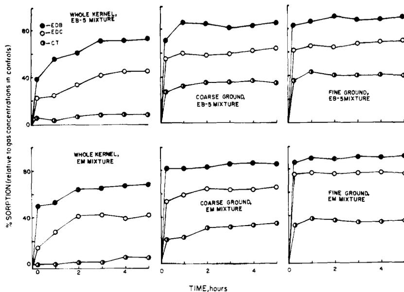
Figure 3. Sorption of ethylene dibromide, ethylene dichloride, and carbon tetrachloride in vapor phase at 27° C. by Selkirk wheat of 9.0% moisture content of three particle sizes and after two treatments
