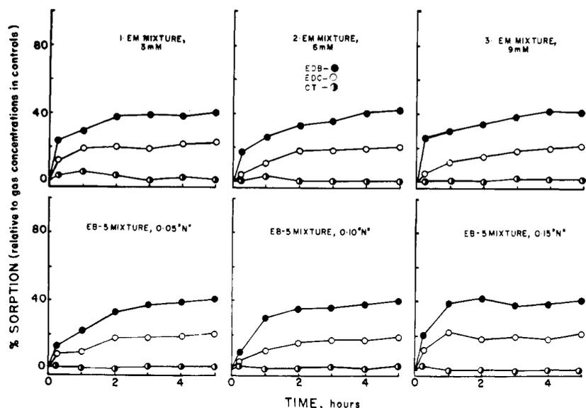
Figure 5. Sorption of ethylene dibromide, ethylene dichloride, and carbon tetrachloride in vapor phase at 27° C. by whole-kernel Selkirk wheat of 13.5% moisture content after application of (upper) EM (equimolar) mixture at dosages of 3, 6, and 9 mmoles and (lower) EB-5 at dosages of 0.05, 0.10, and 0.15 N
