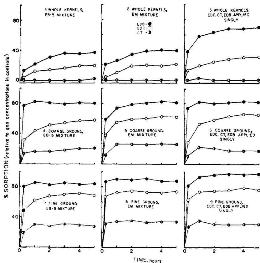
Figure 2. Sorption of ethylene dibromide, ethylene dichloride, and carbon tetrachloride in vapor phase at 27° C. by Selkirk wheat of 13.5% moisture content of three particle sizes and after three treatments
