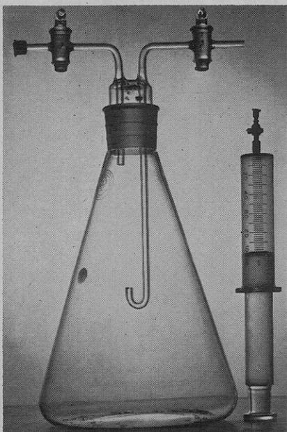
Figure 1. Strand flask containing ethylene dibromide, ethylene dichloride, and carbon tetrachloride gas mixture and 100-cc. precalibrated hypodermic syringe used as micro fumigation chamber
